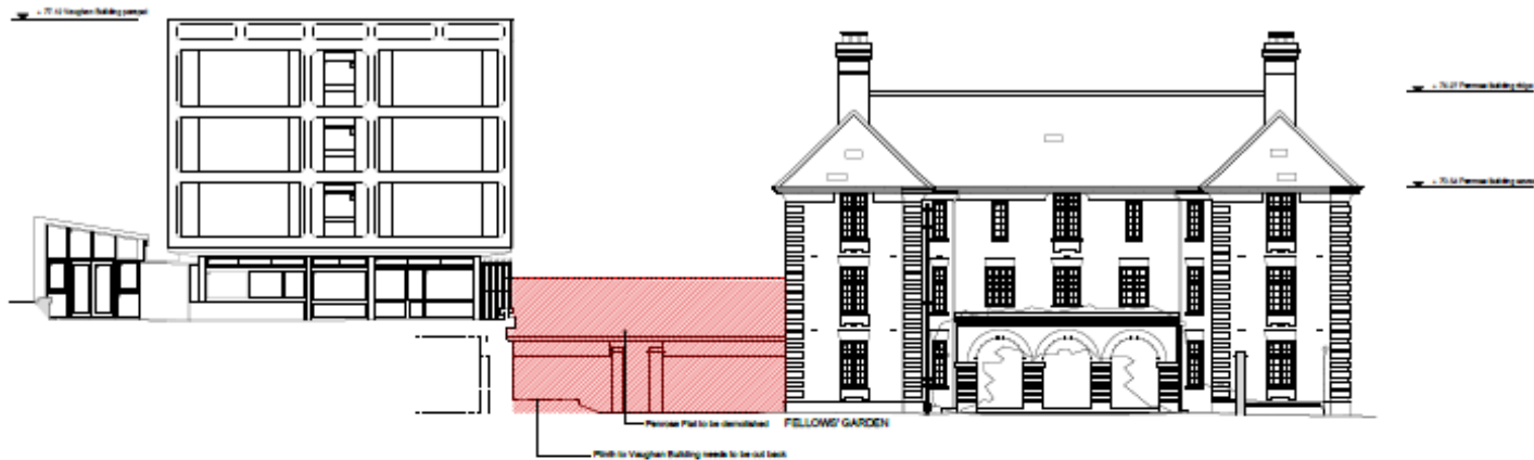
01 Existing East Elevation
